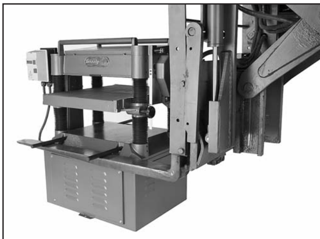
Figure 6. Example of planer being lifted using forklift.
